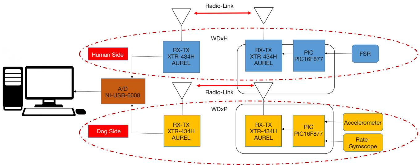
**Figure 2** The architecture of the *telemetric system*.
